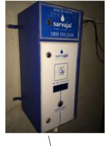
GPRS device to connect Water ATM to cloudbased software
